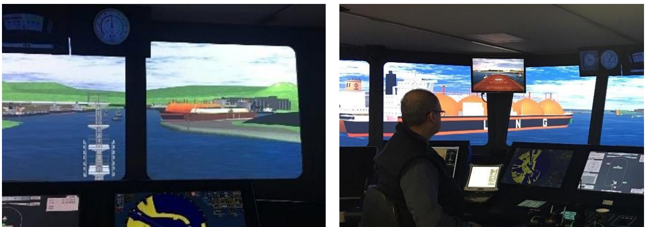
Figure 1: (Left) Arrival through The Cut showing the bow of the LNGC protruding limiting the view of the Inner Harbour. (Right) Departure from Berth 102 showing reduced visibility of The Cut due to the bow of the LNGC
