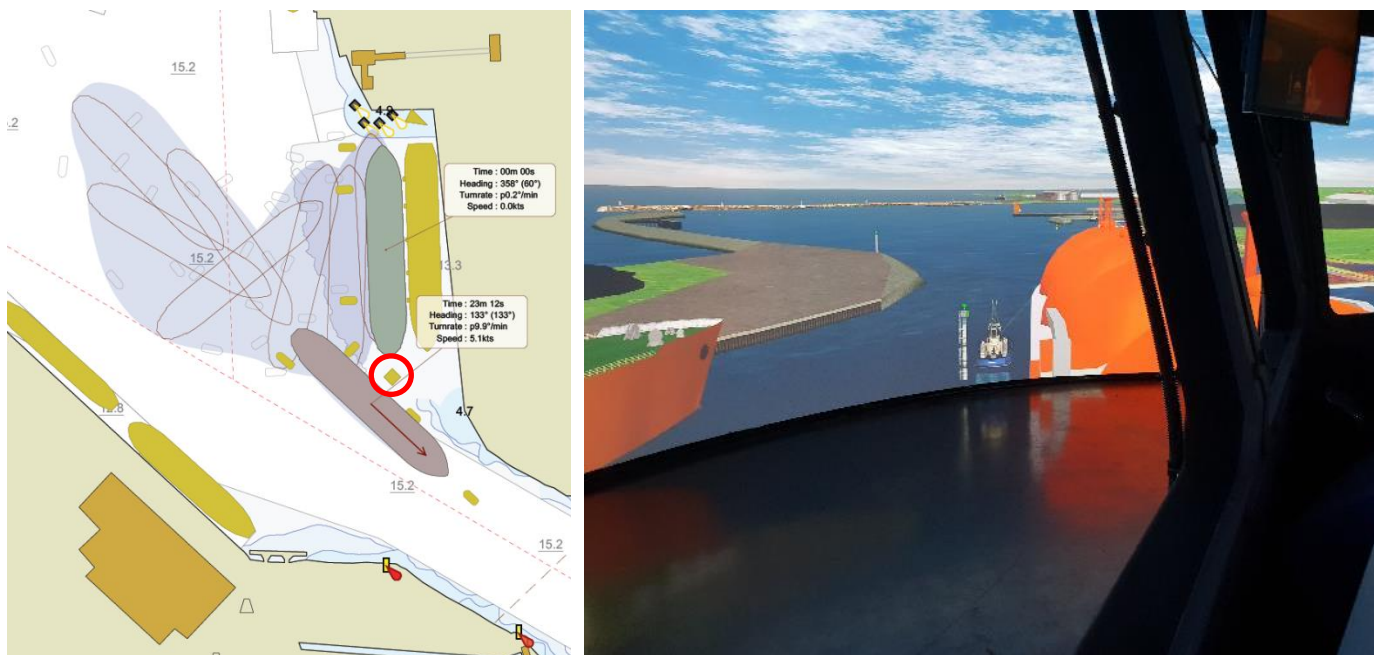
Figure 2: LNGC departing Starboard-side-to in a 25 knot SW wind which was deemed a failure due to clearance to the navigational marker highlighted in red.
